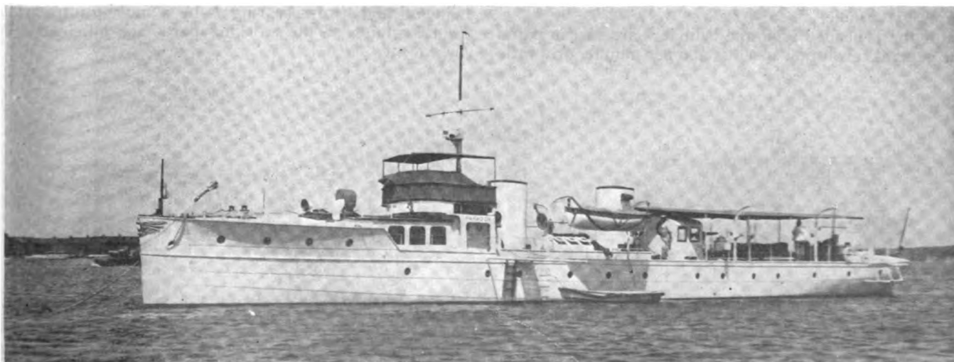
Paragon. Mr. Chas. J. Davol's New 120-Ft., T. B. D.-Type Motor Yacht. She is Driven by a Six-Cylinder, 9 In. by 14 In. Winton Gasolene Engine
