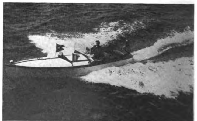
White Rat, a 20-Ft. V-Bottom Runabout at Thousand Islands, N. Y., Equipped with a Sterling Engine Which Gives Her a Speed of 22 Miles per Hour
