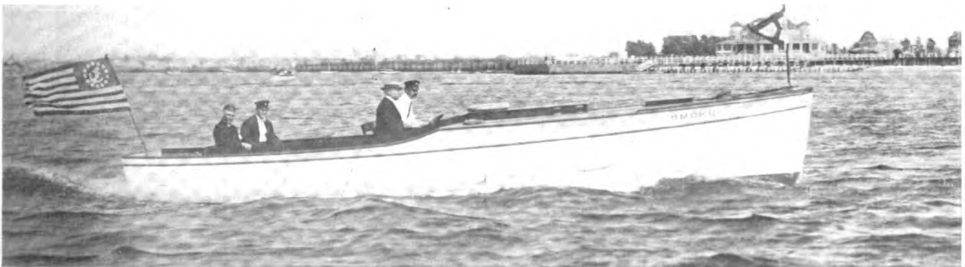
Smoke. Length Over All 32 Ft., Breadth 7 Ft., Draught 2 Ft. 8 In. Power 4-Cylinder 4\frac{1}{2} In. x 5\frac{1}{2} In. 20-30-H.P. Sterling Engine. Speed 13 Miles per Hour. Allerton & Brophy, Owners. Designed by John R. Brophy
