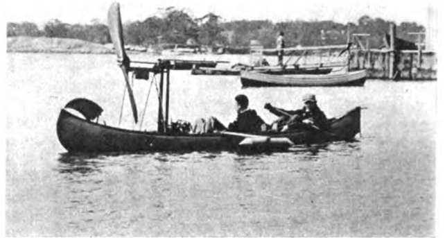
A Canoe Fitted with an Air-Cooled Motor Driving an Air-Propeller. While Not a Practical Mechanical Proposition Much Fun can be Derived from a Boat Thus Equipped
