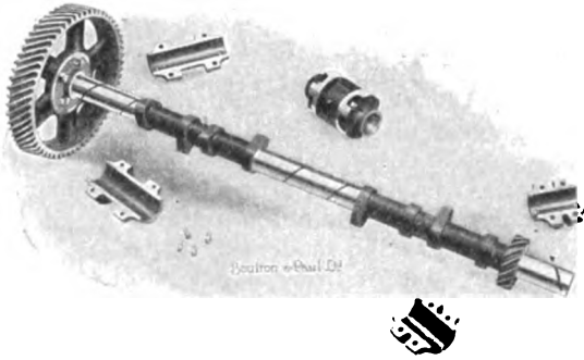
A Cam Shaft. Its Bearings are Built in Halves, and Oil Channels are Cut in the Shaft
