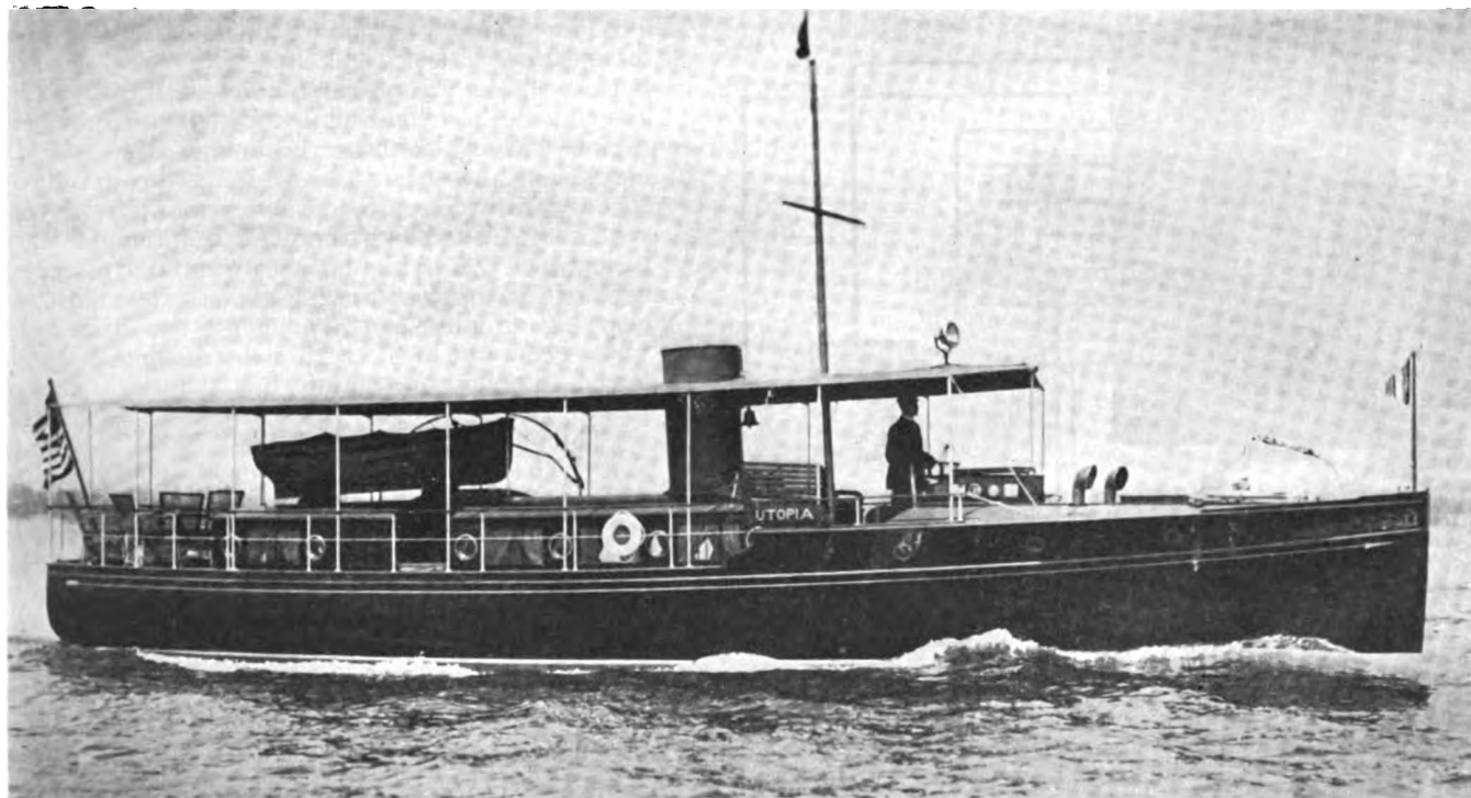
Utopia, a 50 Ft. by 10 Ft. 8 In., Bridge-Deck Cruiser. Built for Mr. Conrad Stein by the Luders Marine Construction Co., of Stamford, Conn., and Fitted with a 35-H.P. Sterling Gasolene Engine. Speed 11½ Miles per Hour
