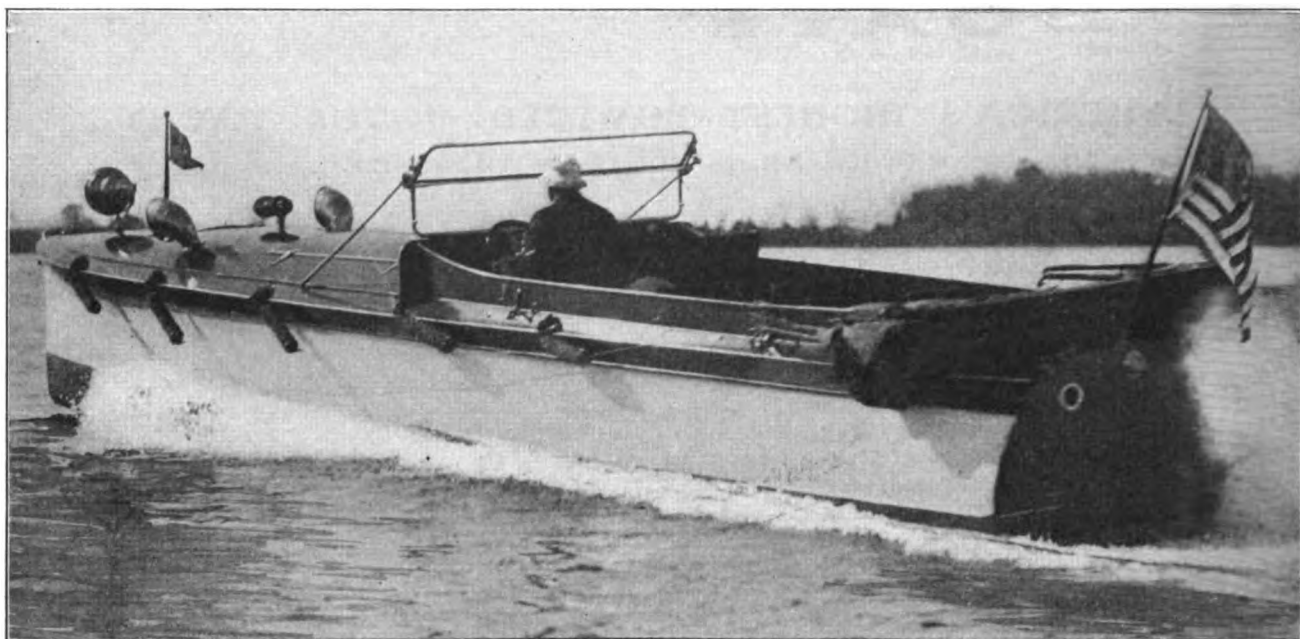
A Thirty-Five-Foot Ramaley Runabout as Owned by Senator D. F. Harding, Jr., of Chicago. She is Powered with Six-Cylinder 100-H.P. Van Blerck Equipped with a Liece-Neville Electric Starter. Speed 32 Miles per Hour
