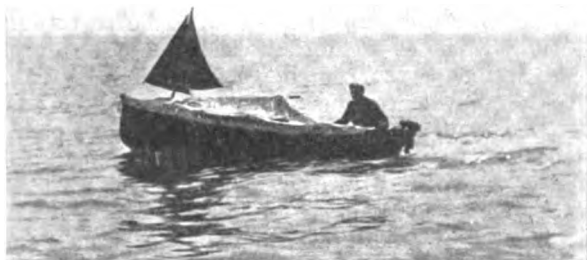
At Times It Was Difficult to See the Sea Pup. So the Sail Shown Above Was Rigged and Was Always Visible Even When the Boat Was in the Trough of the Waves
