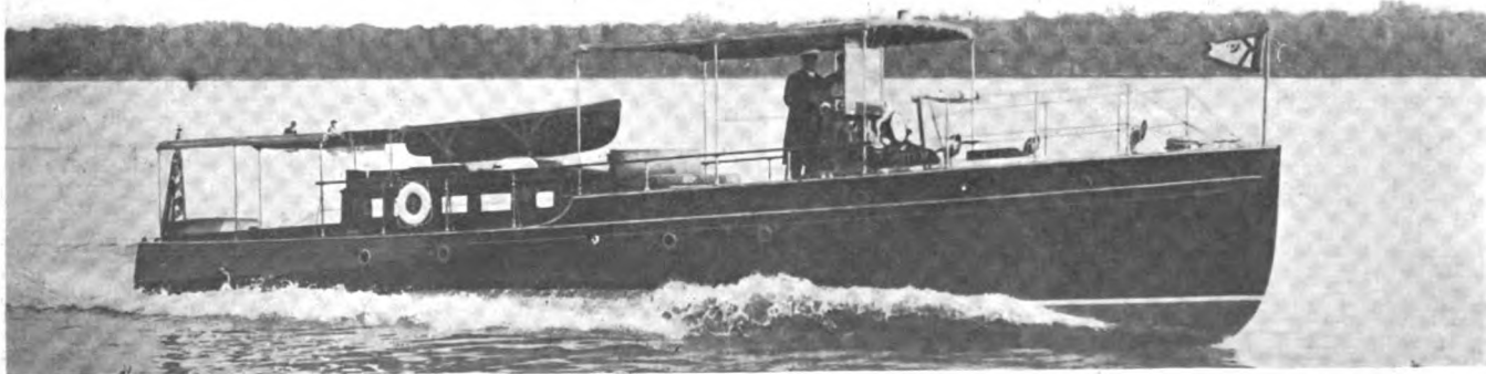
Betty M. a 48-Ft. by 9 Ft. by 2½ Ft., Raised Deck Cruiser. She is Powered with Two Six-Cylinder 100-H.P. Van Dierck Gasolene Engines. Commodore Chas. W. Kotcher, Owner
