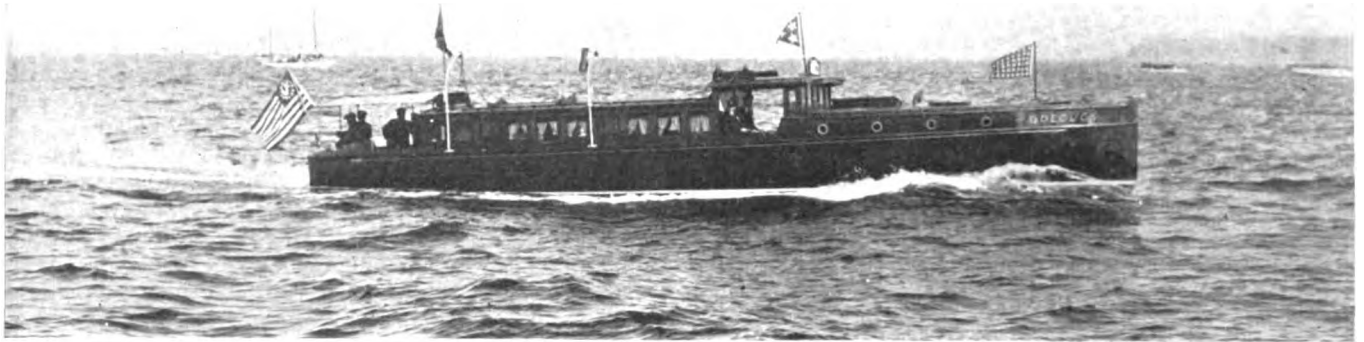
Goeduck, a 59-Ft. by 9-Ft. Cruiser, Owned by Mr. Wm. G. Norris, of Seattle, Who Uses Her on Puget Sound. The Engine is an Eight-Cylinder 100-H.P. Sterling, Which Drives the Little Vessel at 20 M.P.H. When All-Out. At 12½ M.P.H. the Fuel Consumption is 4 Gallons of Distillate Oil
