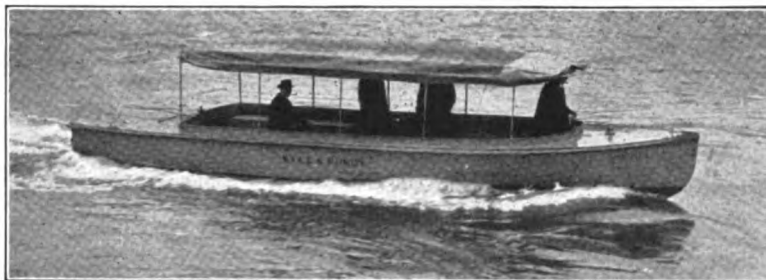
Tunnel Stern River Boat for South America
