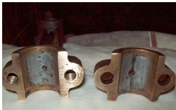
Figure 2 - replacement rod with babbitt material in place
